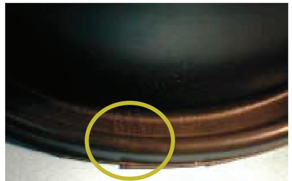
**Definition:** **Strike-through** is the amount of rubber that comes through the fabric to either fully or partially encapsulate the fabric during manufacturing.
