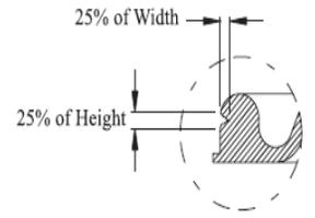
2. Void not to exceed 25% of the height and 25% of the width, simultaneously.
