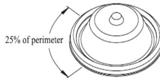
3. Length of void shall not exceed 25% of the perimeter of the part.
