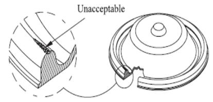
4. Any voids at the top of the bead, which may effect bead height when viewed from side, are unacceptable.
